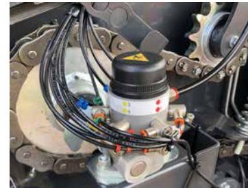
Automatic chain lubrication with individually adjustable outlets.
