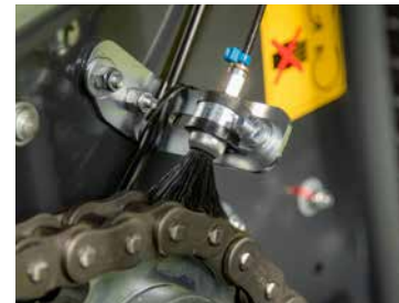
Automatic chain lubrication is standard on FixBale 500.
