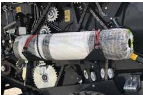
Easy access storage for two spare rolls of net for long working days.
