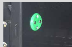
Moisture sensors located inside bale chamber.
