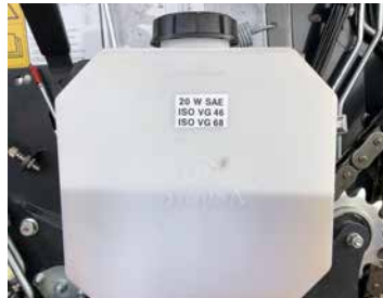
Large capacity chain lube tank.
