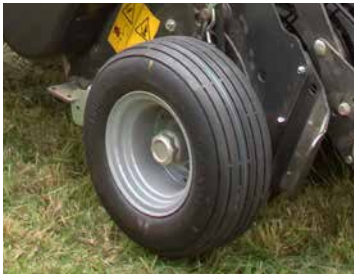
Generous flotation tyres with simple height adjustment.
